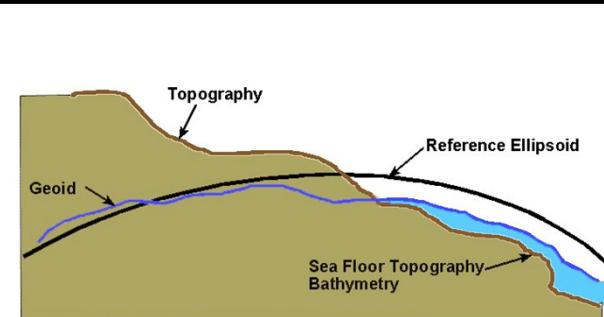
Three Surfaces of Geodesy
